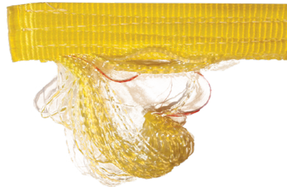
TENSION BREAK / LOOSE THREAD
