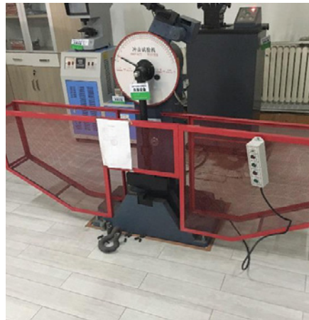
LOW TEMPERATURE IMPACT TESTING
