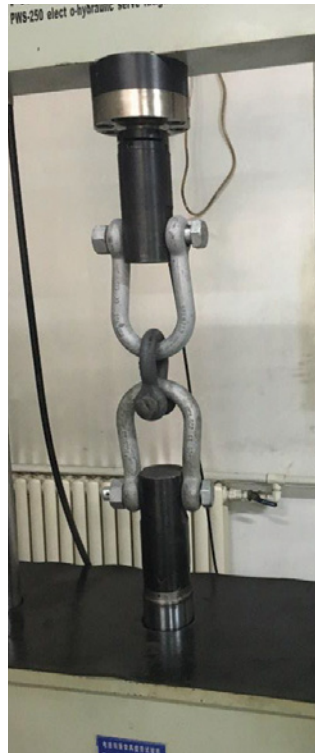
CYCLE TESTING - 20,000 CYCLE MINIMUM
