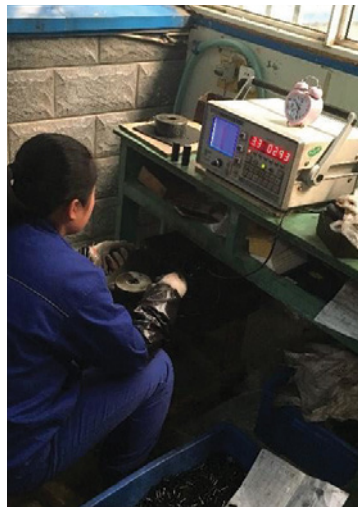
LOAD PIN CRACK DETECTION AND INSPECTION
