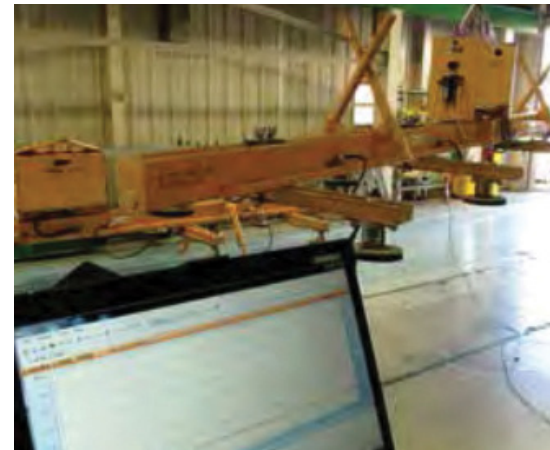
MOBILE VACUUM LIFTER TESTING
