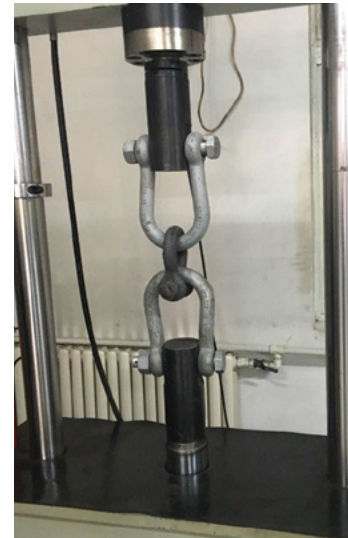
CYCLE TESTING - 20,000 CYCLE MINIMUM
