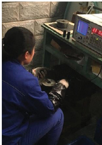
LOAD PIN CRACK DETECTION AND INSPECTION
