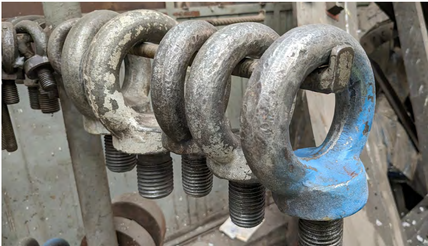
SHOULDER PATTERN LAG SCREW EYE BOLT
